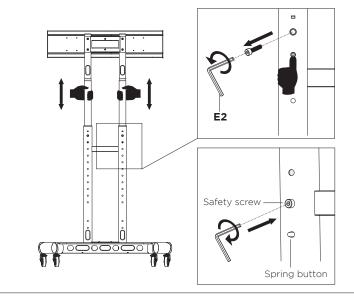
9.2 Person "A" holds the top section of the telescopic column. Person "B" unscrews 2x safety screws from left and right poles by using 6mm Allen key. Put screws aside. Carefully depress both spring buttons on poles by using thumbs, so that person "A" can move top of column down or up to desired height.
