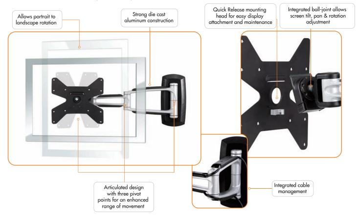
Supports 75x75, 100x100, 200x100 & 200mmx200mm VESA hole patterns. Also supports 200x300, 200x400, 300x200, 300x300, 300x400, 400x200, 400x300 & 400mmx400mm via optional adaptor accessory Product information, single unit
