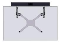
**2)** PMA Kit attached to an X-style (or H-Style) VESA mount with the bar above the display.
