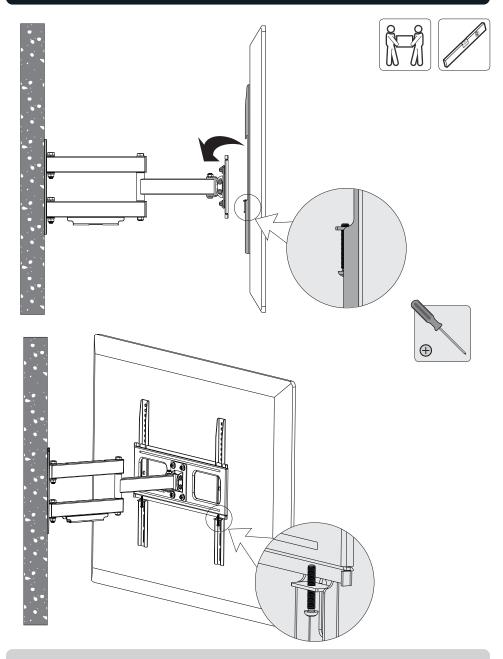
Make sure adapter brackets have been securely hooked onto the wall plate before releasing the TV.
