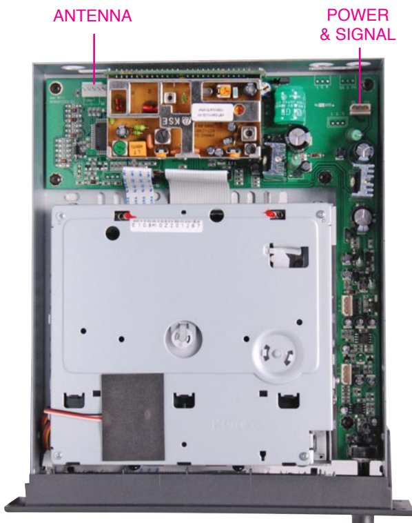
Figure 1: Location of antenna and power/signal headers.
