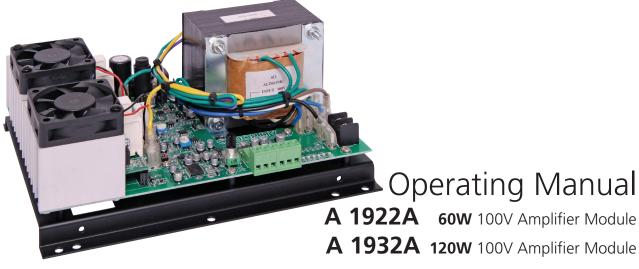
This module is designed for use in emergency evacuation systems and is powered by an external 24V DC source. It accepts a line level audio input and produces a 100V line output via a transformer. It also features short circuit, overload and thermal cutout protection, and is constructed on a steel chassis. Designed with reliability and robust performance in mind, it is the ideal audio power source for evacuation systems, or any application which requires a DC powered 100V line amplifier.
