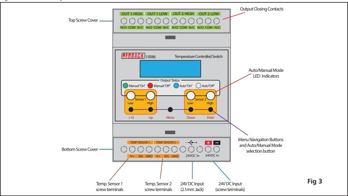
POWER: The unit can be powered by 12V or 24V DC, although a 24V DC plugpack is supplied. Connection can be made via the 2.1mm DC jack or screw terminals. These two inputs are connected in parallel inside the unit, so either could be used as an input, while the other could be used as a 24V DC output to power another device.
