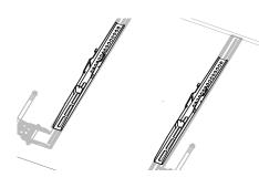
Optional: If your TV mounting rails do not fit inside the soundbar bracket rails (or your TV mount is the flat plate style), add mounting shims between the brackets to give a solid / flat mounting surface for the TV mount.
