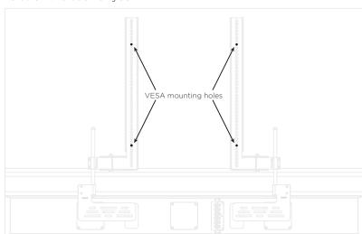
Add your TV wall-mount brackets. The soundbar bracket rails are designed so that most wall-mount brackets will fit inside the rails.
