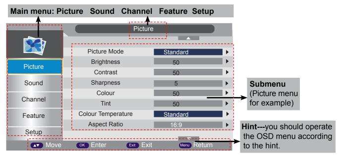
Use  $\land / \lor$  button to select the main menu, and press > / OK button to enter the submenu. In the submenu, use  $\land / \lor$  button to select the function item, press > / OK button to enter the setup menu, then press < / > button to adjust, or press  $\land / \lor$  to select and press OK / < / > button to confirm.
