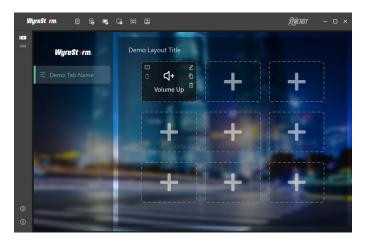
Once you've supplied a name for the button, proceed to select a suitable icon for it. Then, choose the specific device to which you intend to send commands. Following this, define the command itself. Once these steps are completed, click the "Save" button. This action will result in the button being showcased within the workspace for your configuration project.
