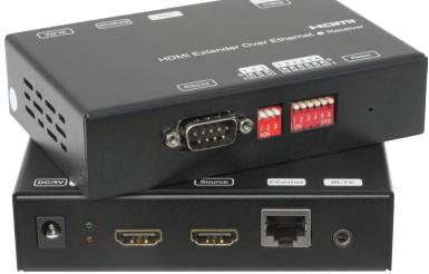
HDMIIPECO uses H.264 as compression type, which takes lower bandwidth and transmits the signal over the LAN more smoothly. It transmits the HDMI signal for up to 120m over single cat5e/6 cable at point to point, as well as point to many and many to many over Ethernet switch. It can be widely used in various locations, such as meeting room, class room,metro, airport, home, mall advertisement...etc.
