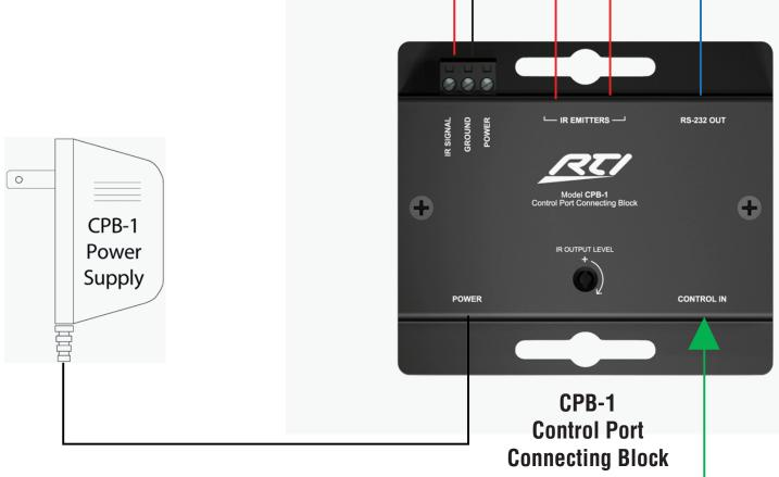
The Control Port from any RTI keypad can be connected to the CPB-1 to control one device via RS-232, as well as allow for additional control via infrared.
