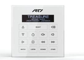
The WK2 Water Resistant In-Wall Controller has a clean, sleek design with an all glass exterior that is perfect in locations such as bathrooms. The solid state glass keypad utilizes capacitive touch for the fourteen programmable buttons. A bright OLED display provides two-way feedback for fast, intuitive control when used with an RTI XP series control processor.
