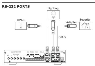
The XP-6s is capable of two-way control using RS-232 communication via three RJ-45 output ports using standard Cat-5 cable with RJ-45 termination (568B). The XP-6s ships with three RJ-45 (female) to DB-9 (male) adapters.
